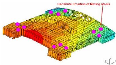
Figure 5.5: Deck box hogging when resting on barge
