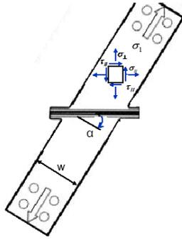
Figure 3.9: Example of weld with inclined principal stress direction
