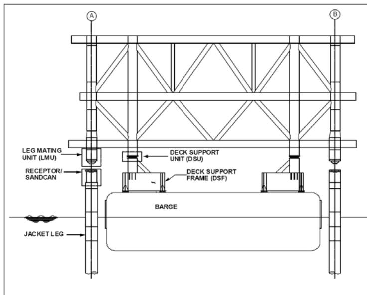
Figure 5.4: Location of Float-over Hardware Components
