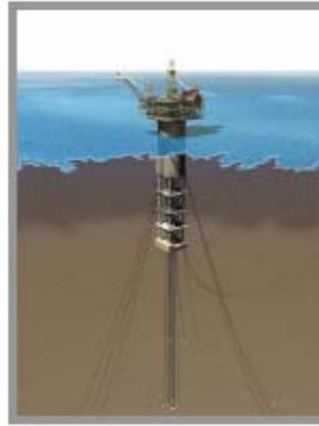
Figure 3.2: Typical truss-spar Arrangement
