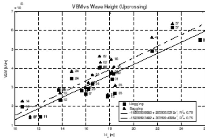
Figure 3.3: Correlation between hogging and sagging peaks and the height of abnormal waves
