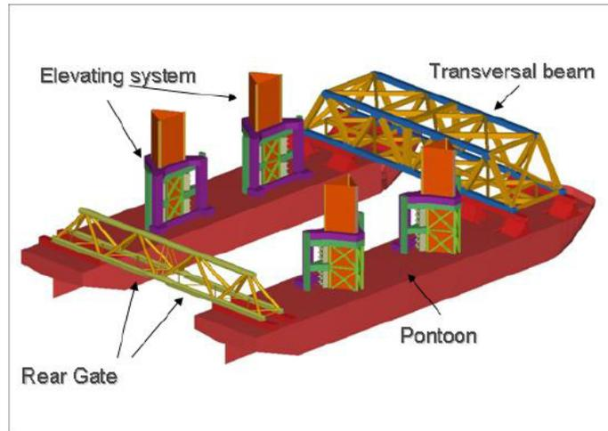
Figure 5.8: Main Structural Parts of the DSIVSystem
