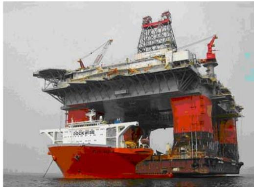
Figure 5.11: Jumboised Blue Marlin transporting the 59,500 t heavy Thunder Horse PDG platform
