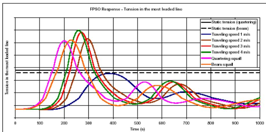
Figure 3.4: FPSO response to a forward travelling front
