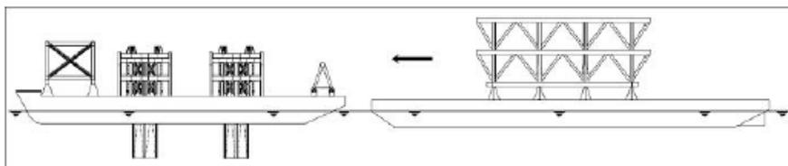
Figure.5.10: Topside load out from barge onto DSIV
