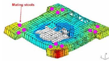
Figure 5.6: Deck box sagging when resting on mating stools
