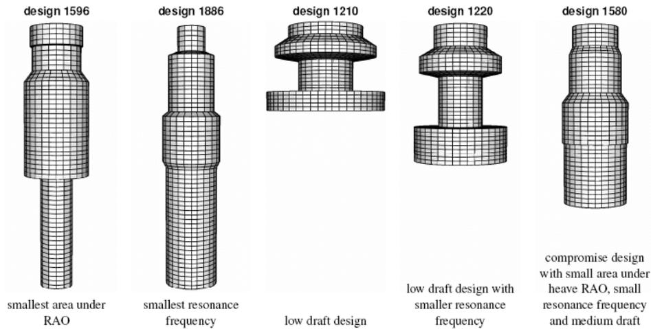
Fig.3.13: Example of spar hull optimization results, using various criteria (Birk and Clauss 2008).
