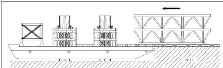
Figure 5.9: Topside load out from quay onto DSIV
