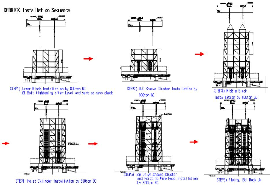
Figure 5.1: Dual Hosting Tower Installation Sequence
