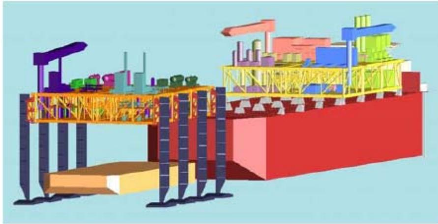
Figure 5.2: “Jack-Deck” Installation Concept
