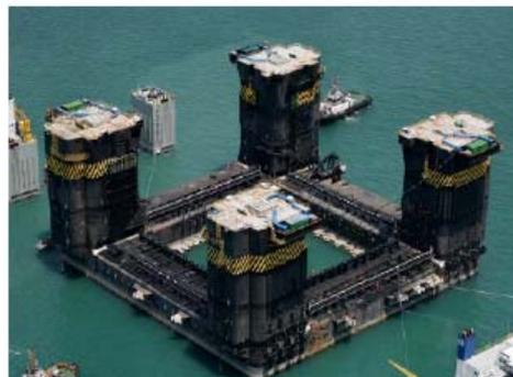
Fig. 3.12: Hull structure of the new generation of floating platforms
