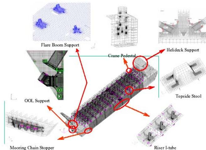
Figure 3.10: FE model of global FPSO and specific details
