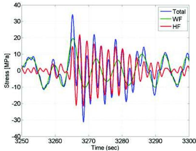
Figure 2. Stress measurements amidships on a large container vessel in a high sea-state. Direct wave-induced stresses on the rigid hull (WF), slamming-induced whipping stresses (HF) and the total combined stress, Andersen (2014).
