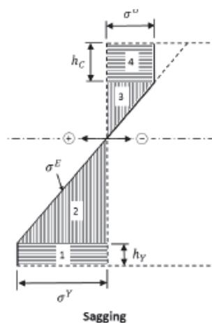
Figure.1 Assumed stress distribution at ultimate strength in sagging in a simplified method
