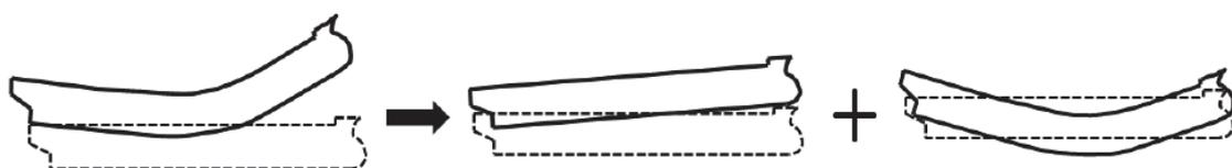
Figure 1.5 Decomposition of displacements (rigid body motion and elastoplastic components) [5].
