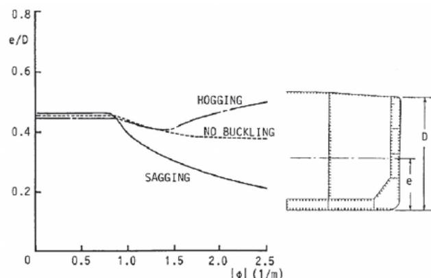
(b) Shift of neutral axis in cross-section
