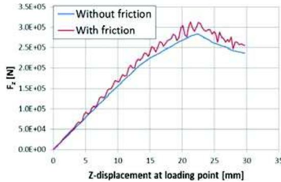
Figure 3 The comparison of calculated load displacement curves between with/without friction forces.
